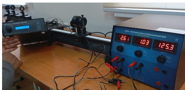
5-rasm. LED ga kuchlanish berilganda undan tok oqib o'tishi va uning quvvatini o'lchash.
