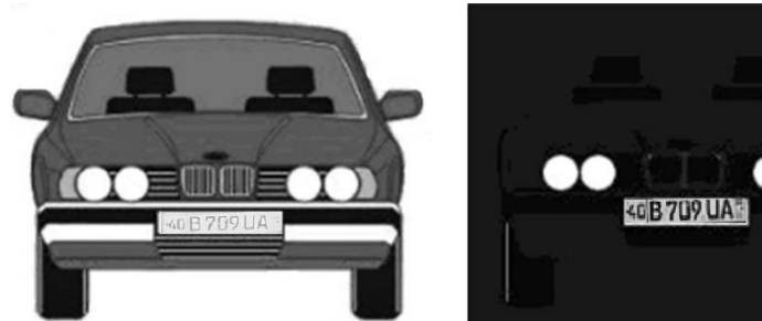
Fig. 2 Image preprocessing: a) original image, b) using IR illumination, c) binarized image
