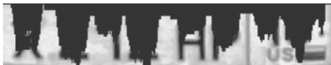
Fig. 2. Histogram of brightness distribution of license plate pixels
